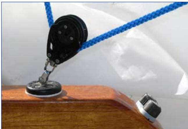
The mainsheet swivel on Thistle 3669 is sturdy and functional, and the medium cam cleat mounted on the aft face of the centerboard trunk gives the driver a free hand for between races. Use a manual ratchet block on the trunk and an automatic ratchet block on the boom.
